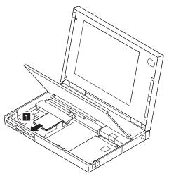
**Warning:** The IC DRAM card is sensitive to physical shock. Incorrect handling of the card can damage it. The eject tape (P/N 53G9318) must be used to remove the card.
